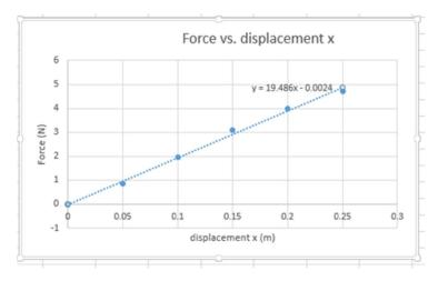
From the equation for that straight line (y = 19.486x - 0.002) we can conclude that the best estimate of the spring constant is: k = 19.49 (N/m), where 19.49 (N/m) is the slope of the line and -0.002 (N) represents the y-intercept.
